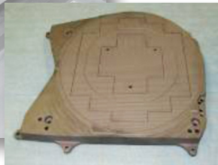
◀ Support for 200 & 300 mm wafers, <2% backside contact, 100 nm flatness per 50 mm 2 area.
